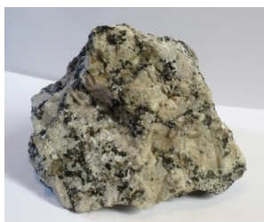
The white and clear crystals in granite are quartz.
